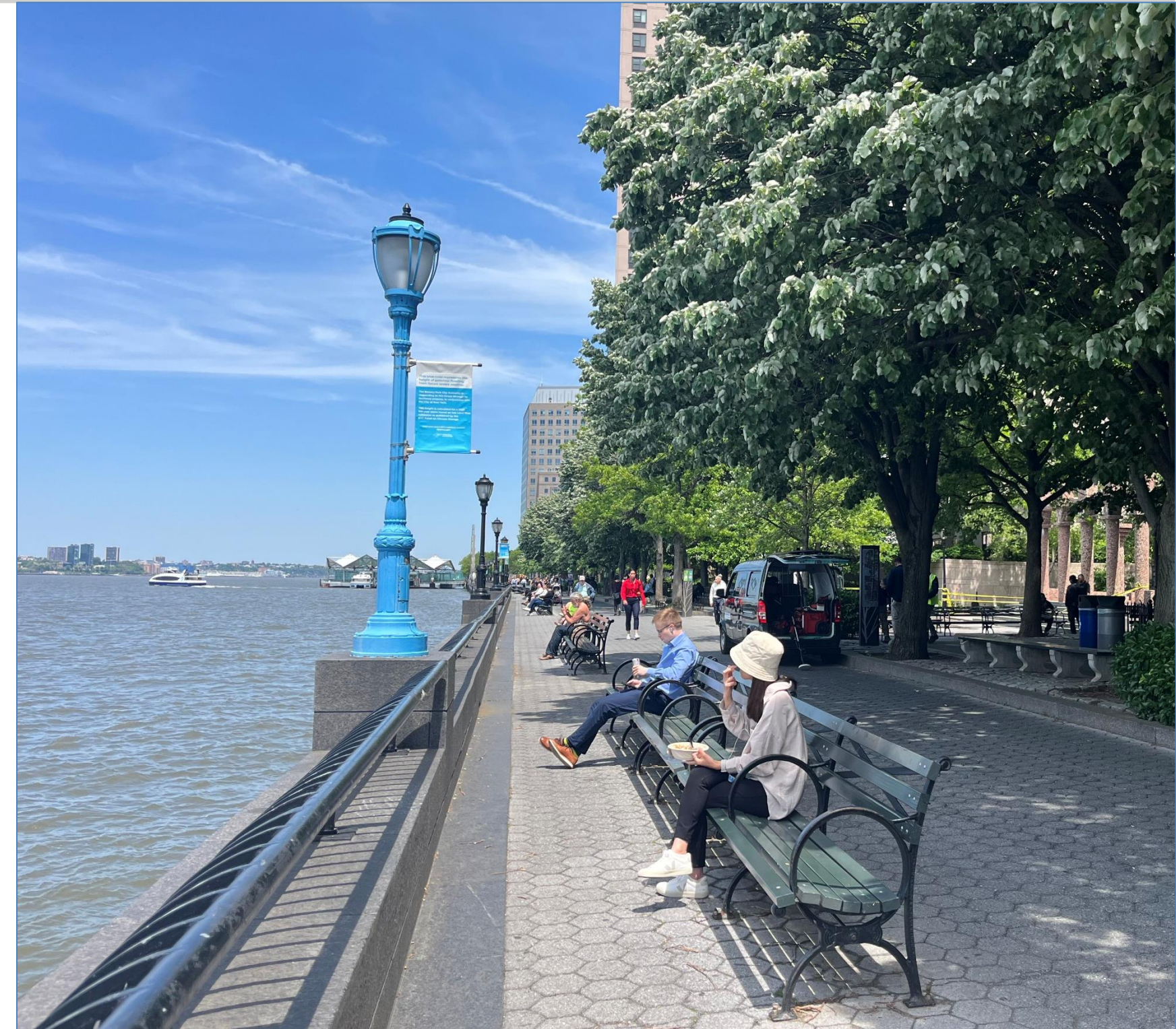
Blue lampposts along the BPC Esplanade illustrate the elevation of storm surge for a projected 2050's 100-year storm, including 2.5 feet of sea level rise. This one at Rector Place is approximately 10.5 feet above the Esplanade
