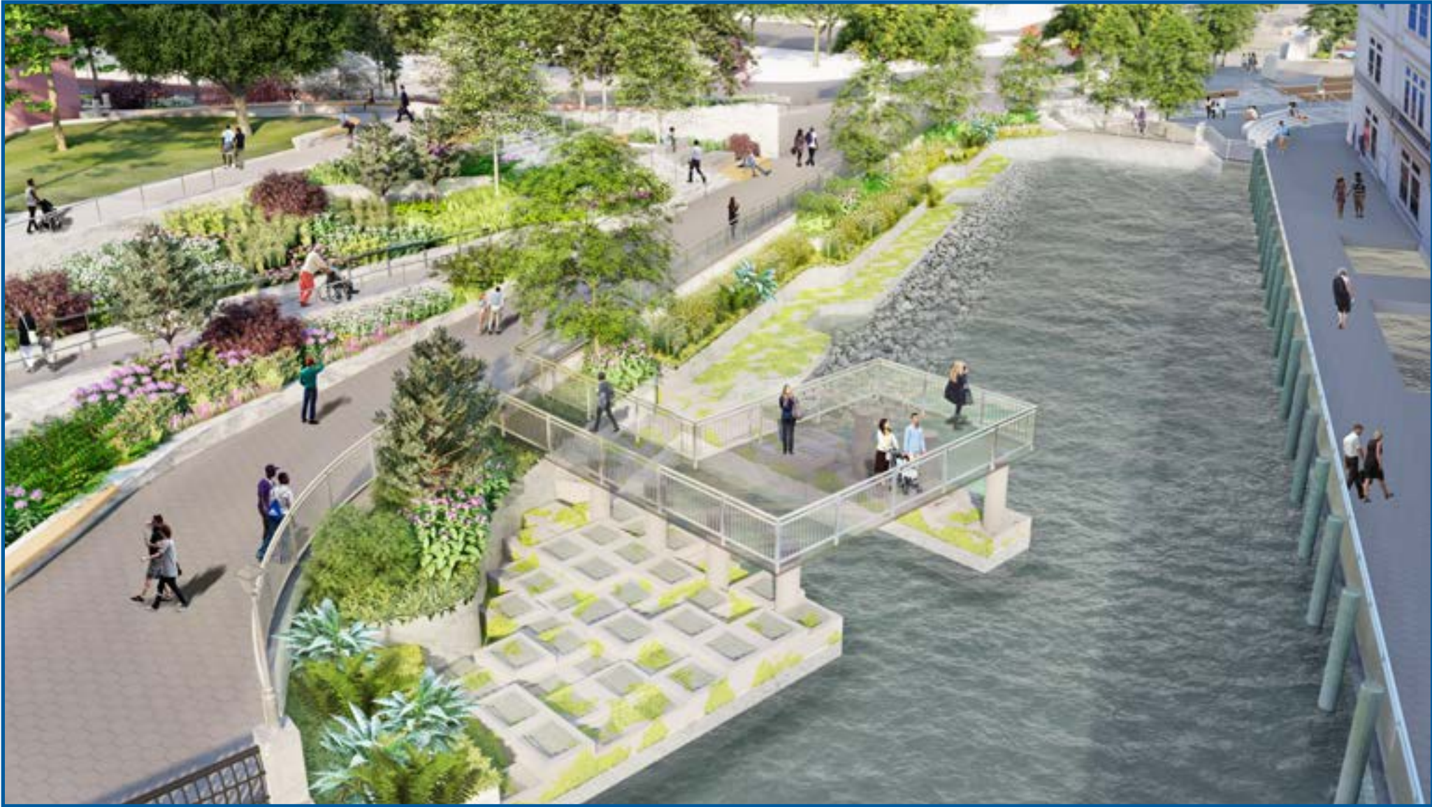
A metal grate viewing platform provides visitors with an educational experience with sight lines to all of the terraces. 50% of available light will pass through to the water below, as to avoid shaded conditions on the water.
