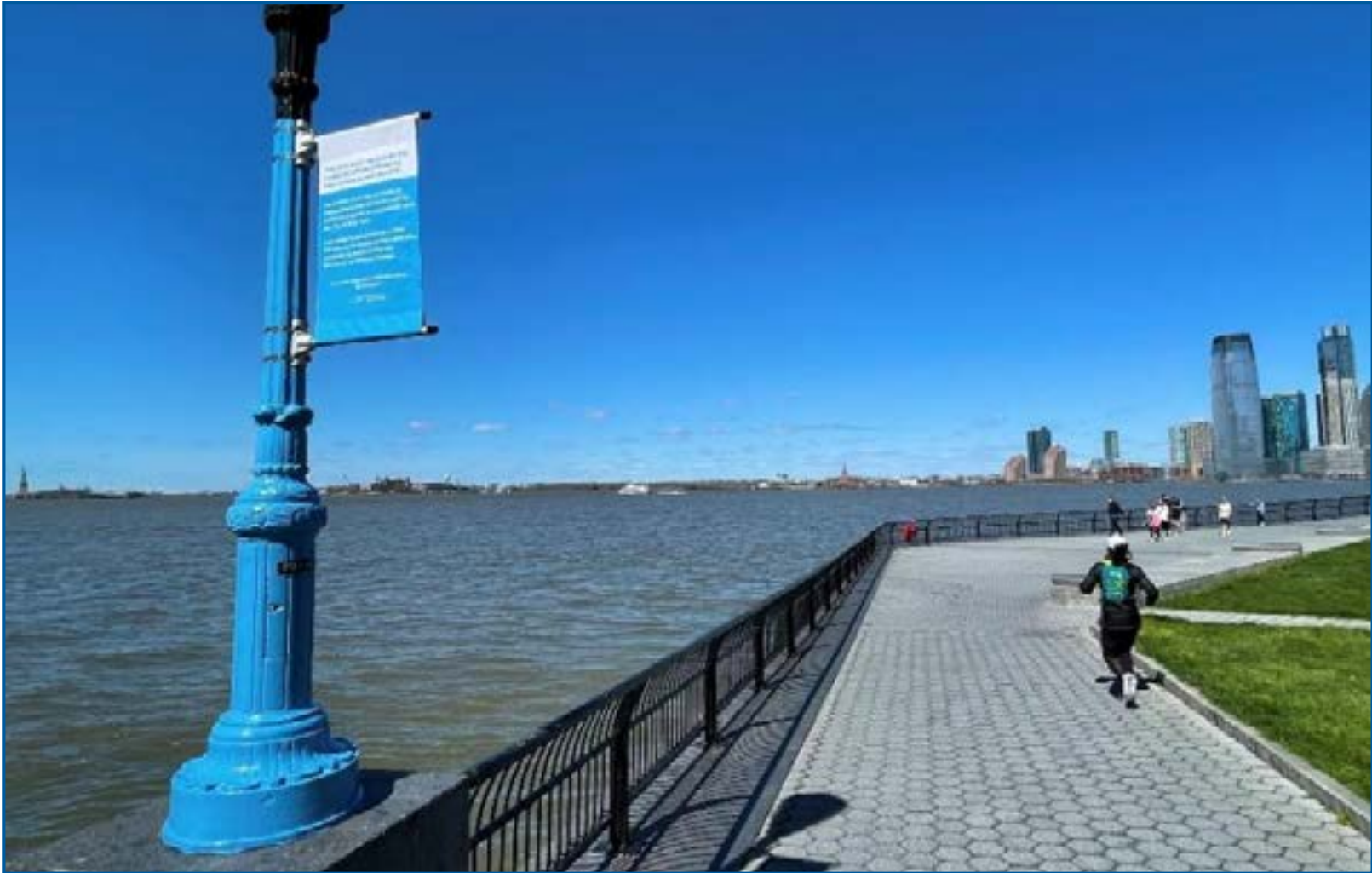
The blue color represents the height of potential flooding from future severe weather. It depicts the height of a 2050's 100 year storm with sea level rise, as published by the NYC Panel on Climate Change
