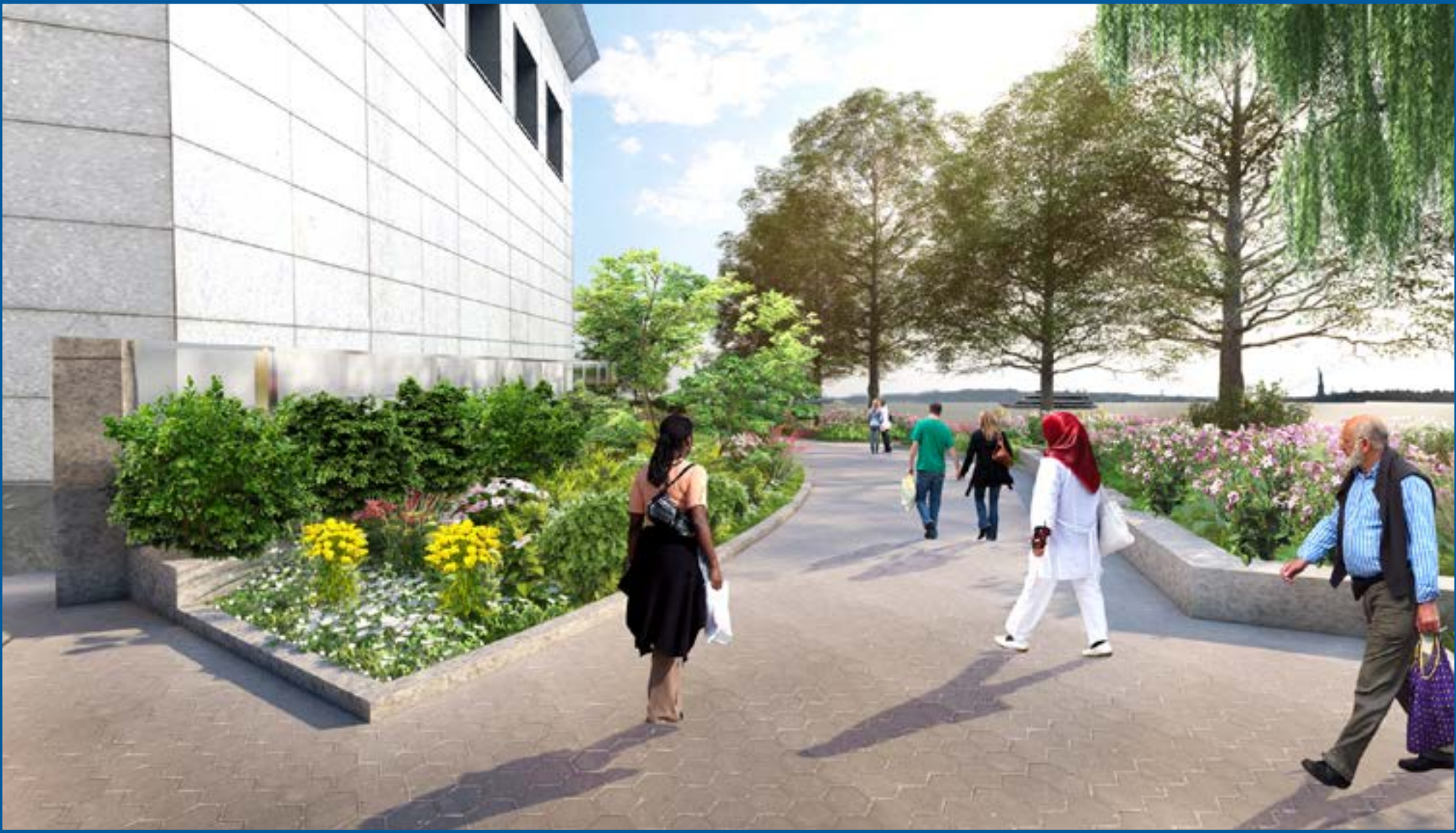
The interior esplanade is re-built in place with new, terraced planters concealing a glass-topped floodwall.
