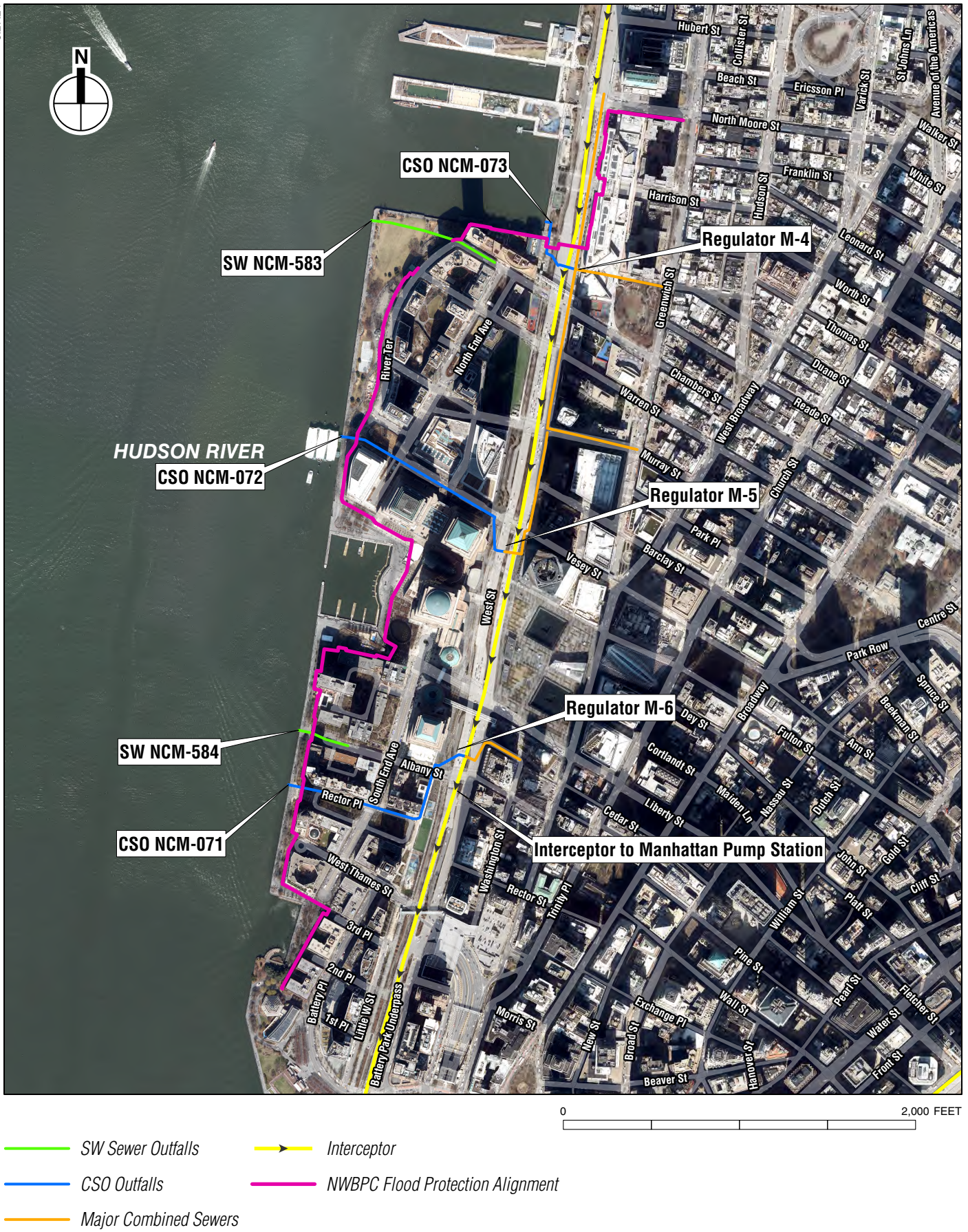
Existing Sewer Infrastructure
