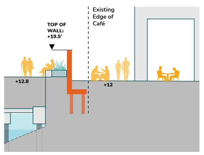
2: Partially Deployable Flood Barrier
