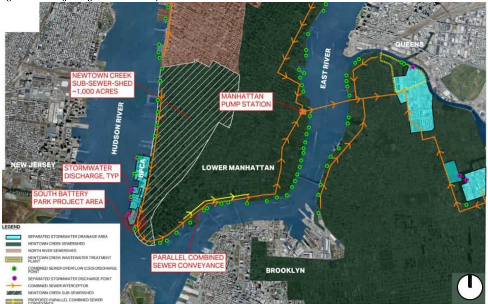
Figure 3.8-2: Existing Drainage to Manhattan Pump Station
